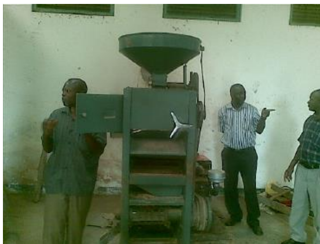
A farmer explaining how the rice huller works.
